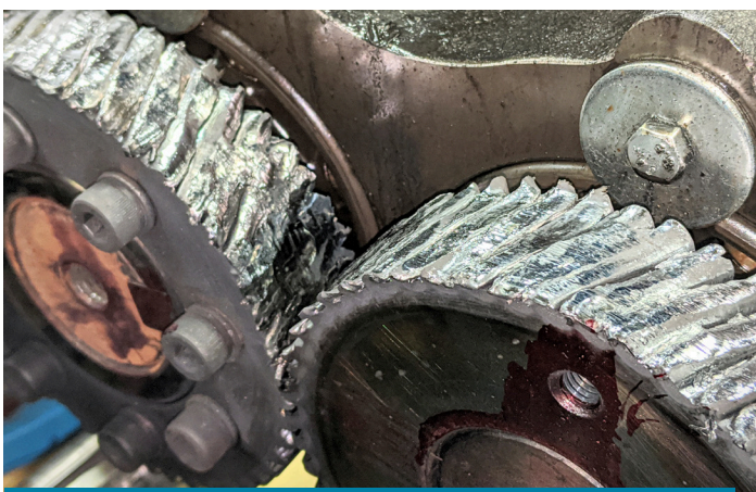
Figure 1 | Example of gear failure from improper lubrication.
