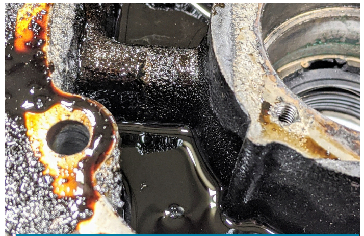
Figure 6 | Example of sludge buildup in oil sump.
