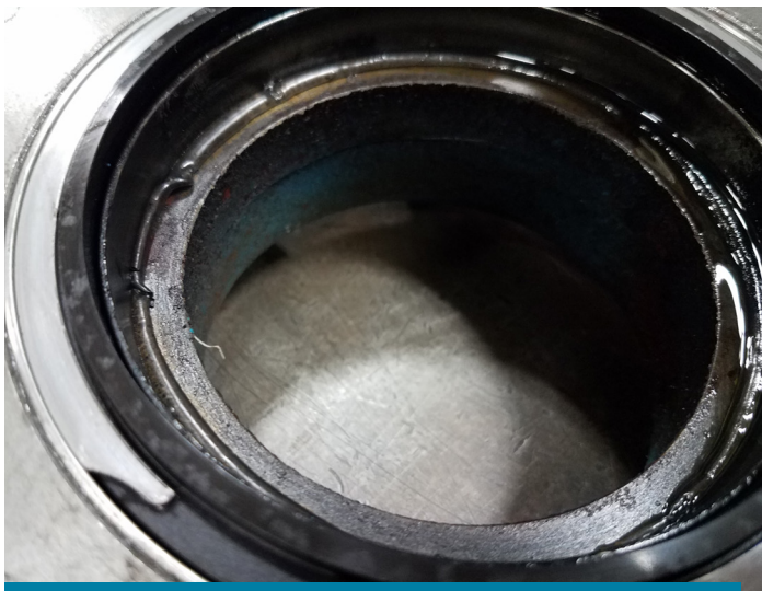
Figure 4 | Example of blistered seal.
